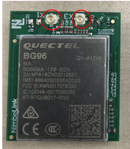
Left: Primary Cellular U.FL connector (X1); Right: GPS U.FL connector (X3)
