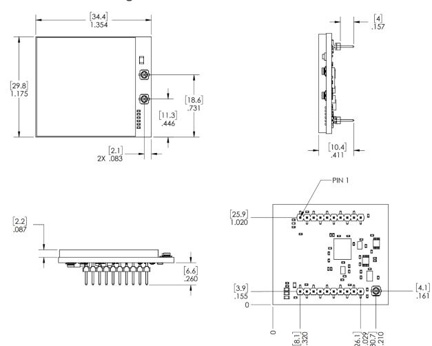
Dimensions are in inches and [millimeters]
