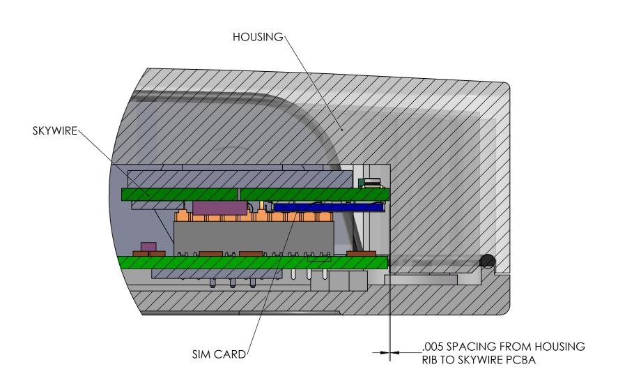
SIM CARD RIB CROSS SECTION
