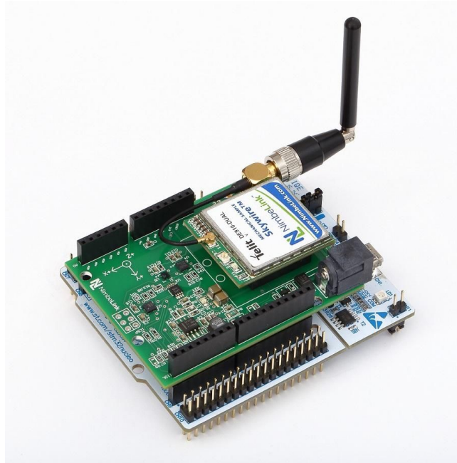
Figure 3-1 Skywire™ ST Micro Shield With Skywire™ 3G EVDO Modem
