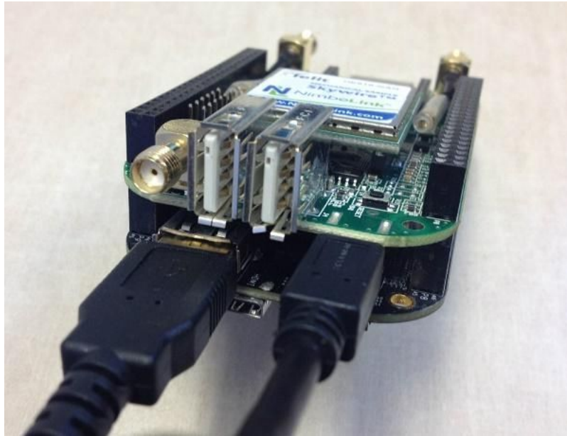
Figure 2-2 Cape to Beaglebone USB Connection
